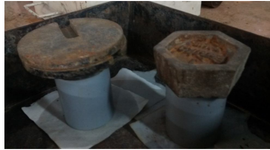
Figure 4. Soil sample in mould with Overburden Pressure for One-Dimensional Consolidation test
